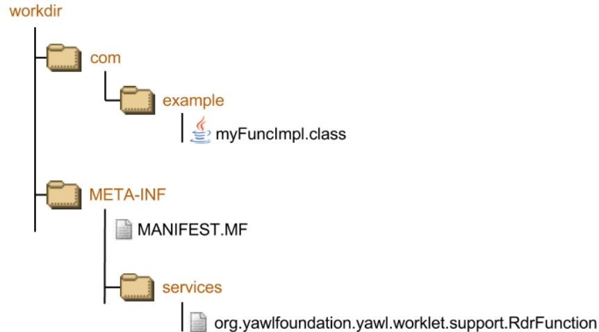
Figure 5.1: RdrFunction implementation JAR structure
